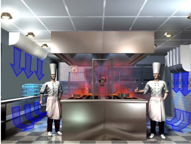
Figure 8 Thermal displacement ventilation, supplying air through displacement diffusers installed at the walls.
